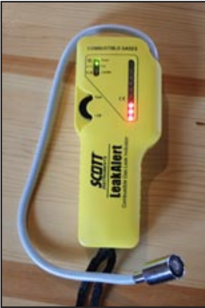
The other piece of equipment I have found most helpful is a combustible gas leak detector.
