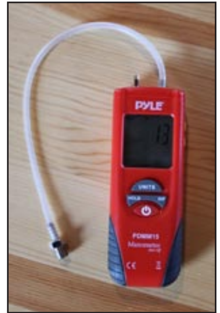
A manometer is a device that can measure very low pressures and specifically in the units of inches of water column.
